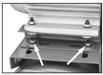
Figure 12. Mounting bolt locations.
